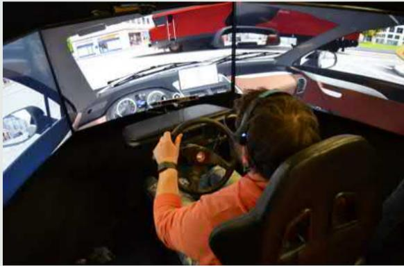
Nervtech's state-of-the-art driving simulator allows us to get driver responses and capture driver's experience as true as in real environment, with the safety of the virtual world.
